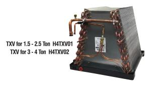
Rifled copper tubing, enhanced aluminum fins. Immersiontested at 500 psi, then nitrogen-pressurized and sealed. Left-hand refrigerant and plumbing connections. Externally mounted flowrater body with Schrader valve. Heavy duty plastic drain pans on all models. AHRI certifiable with certain brands of A/C and heat pump systems. UL listed for use with both R-22 and R-410a when proper metering device is used.
