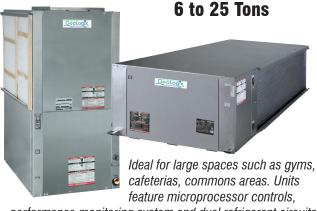
performance monitoring system and dual refrigerant circuits. Available in front or back return, and a variety of discharge locations and voltages. Cabinets are fully insulated and scroll compressors have special double isolation mounting system for quiet operation. **HB Large** capacity models available in horizontal and vertical configurations.
